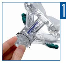
Turn the MicroFit dial to position 24, where the forehead support is fully extended.
